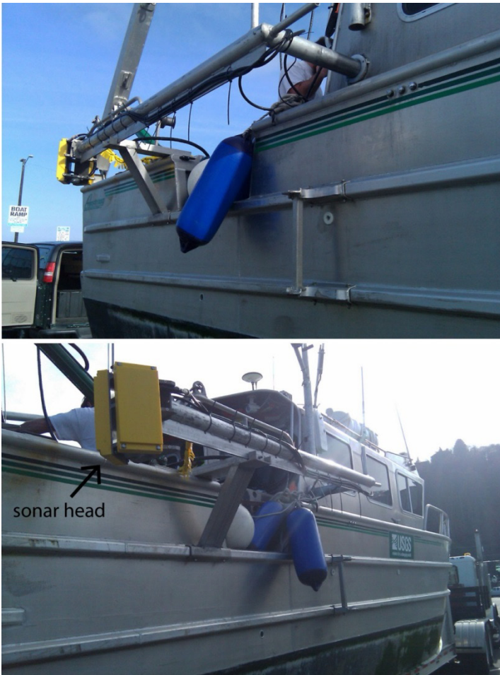
Figure 3. Fore and aft views of the SWATHplus sonar pole mount on the U.S. Geological Survey Coastal and Marine Geology R/V Parke Snavelly .
