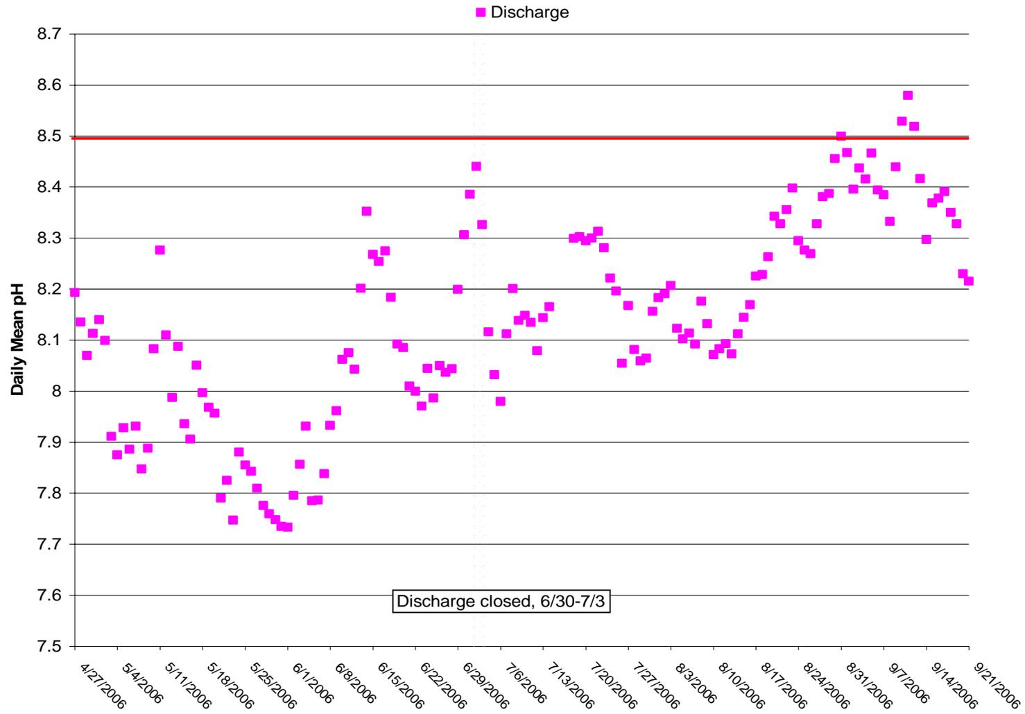
Figure 12a. Pond B2- Daily Mean pH for Discharge and Receiving Water
