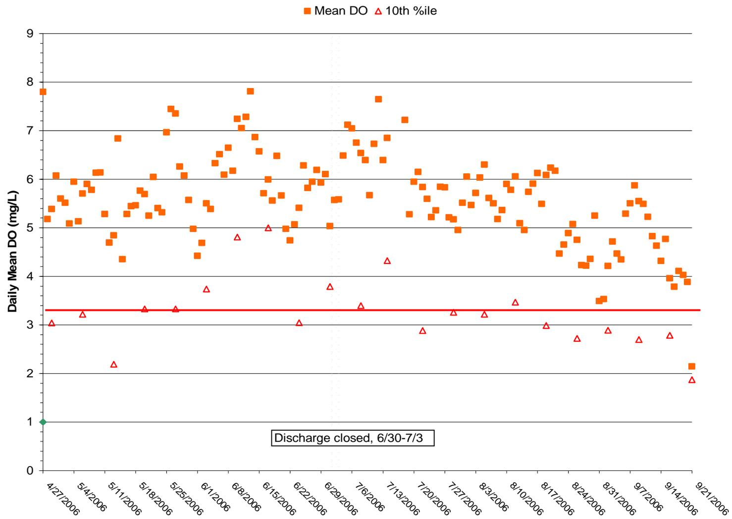
Figure 14a. Pond B2- Daily Mean DO for Discharge and Receiving Water
