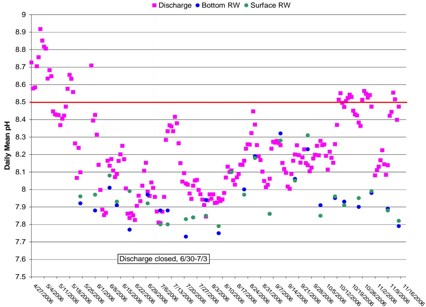
Figure 4. Pond B2C- Daily Mean pH for Discharge and Receiving Water
