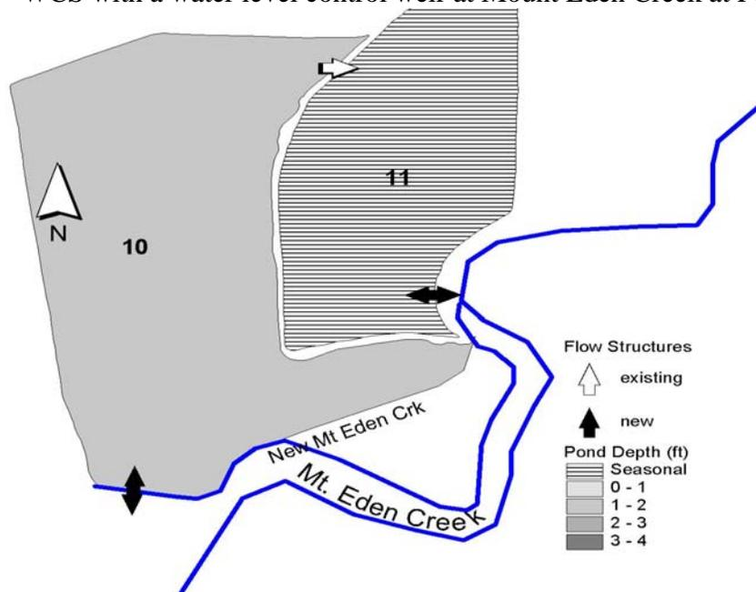
**Figure 1. Map of Ponds and Water Control Structures**
