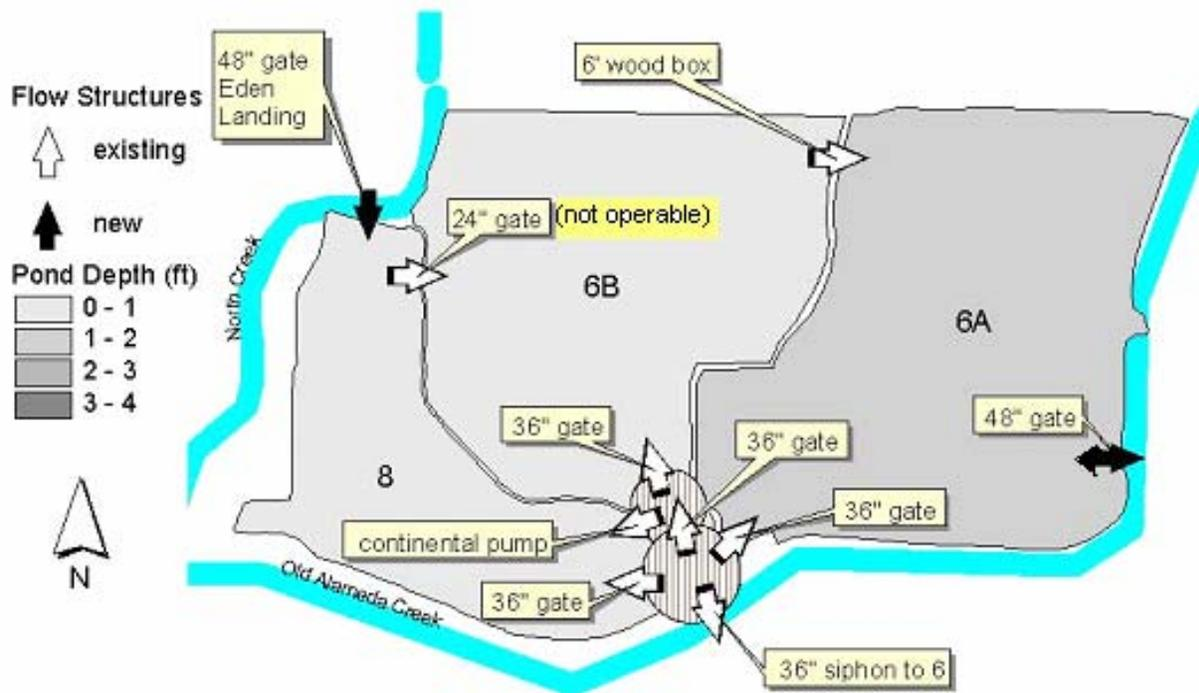
**Figure 1. Map of Ponds and Water Control Structures**
