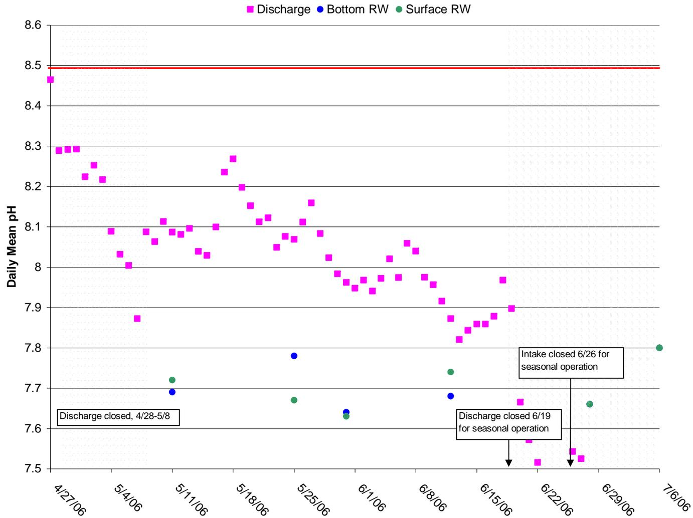
Figure 16. Pond B6A- Daily Mean pH for Discharge and Receiving Water
