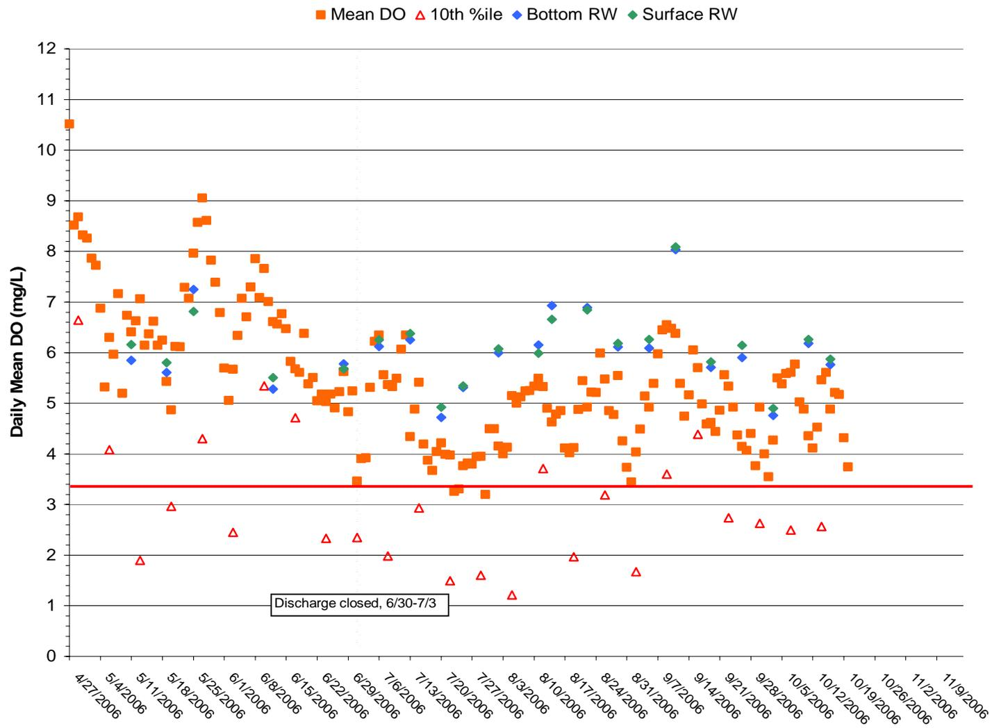
Figure 10. Pond B8A- Daily Mean DO for Discharge and Receiving Water
