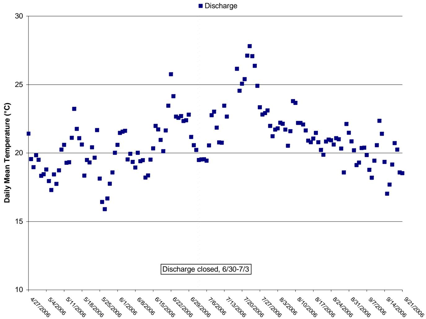
Figure 13a. Pond B2- Daily Mean Temperature for Discharge and Receiving Water
