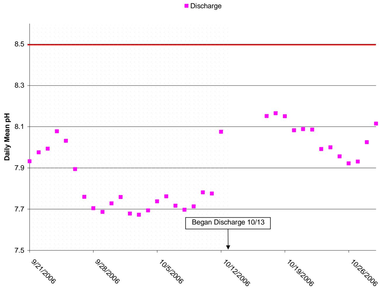
Figure 12b. Pond B1- Daily Mean pH for Discharge and Receiving Water
