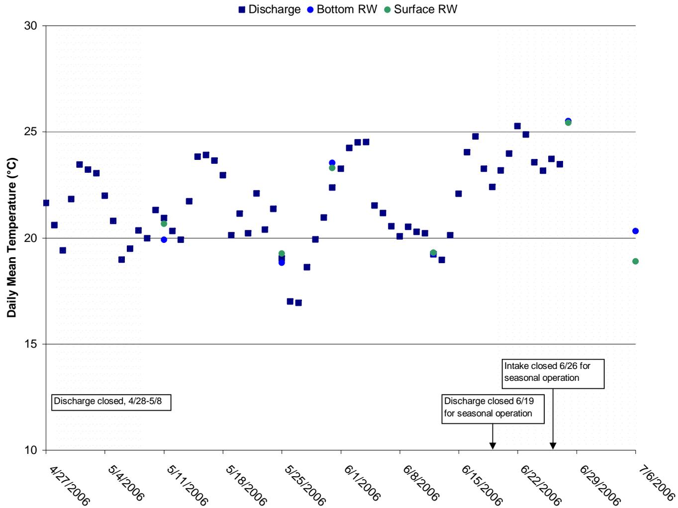
Figure 17. Pond B6A- Daily Mean Temperature for Discharge and Receiving Water
