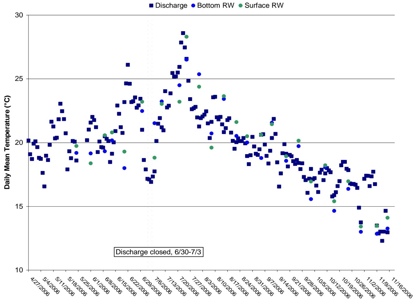
Figure 5. Pond B2C- Daily Mean Temperature for Discharge and Receiving Water
