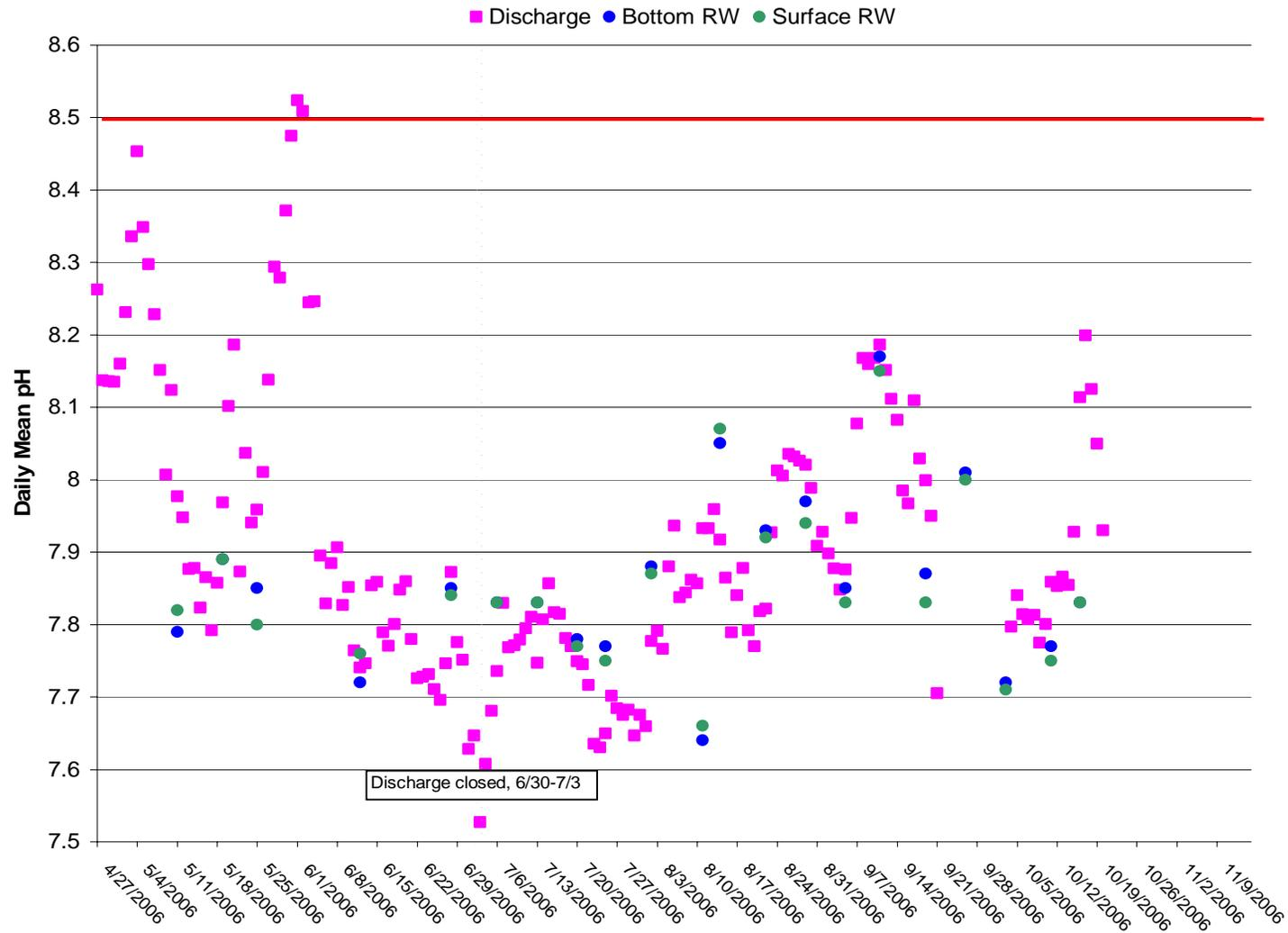
Figure 8. Pond B8A- Daily Mean pH for Discharge and Receiving Water
