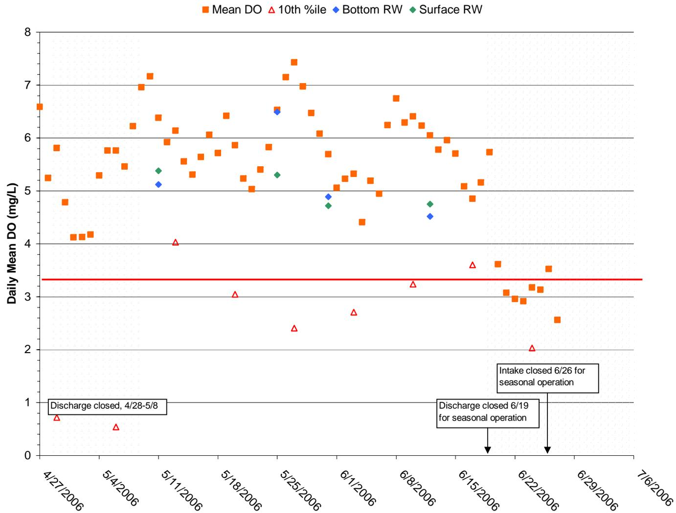
Figure 18. Pond B6A- Daily Mean DO for Discharge and Receiving Water
