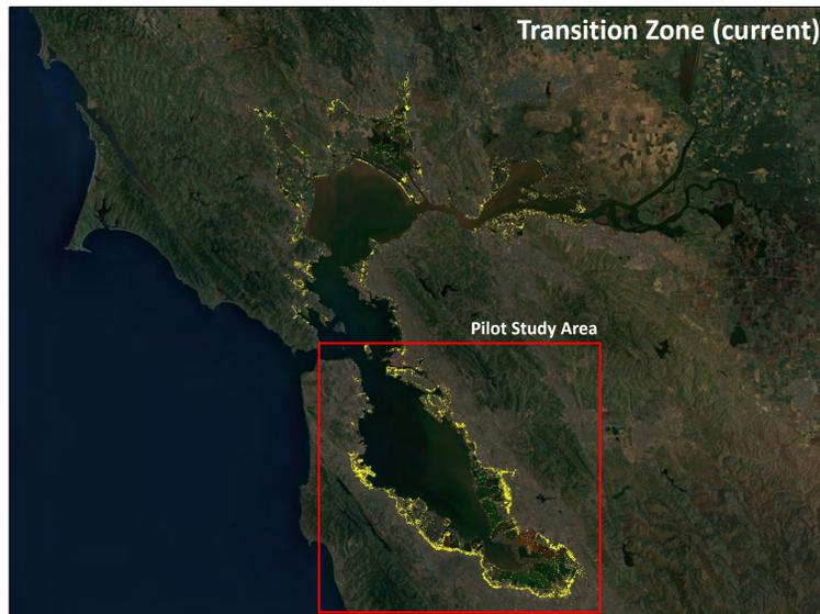
Raster output from the first order model was converted to vector polygons, simplified and adjacent polygons were merged. Final raster results were divided into “tidal and non-tidal” based on “levee on” (tidal) and “levee off” (non-tidal) polygons provided by PRBO.
