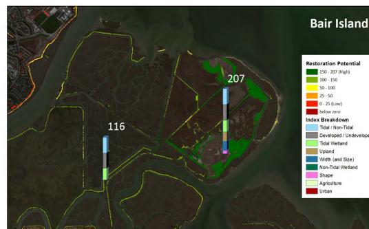
Final Restoration Potential at Bair Island with Index Breakdown comparing restoration potential of two transition zones
