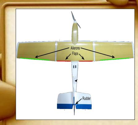
The AggieAir is a multispectral remote sensing unmanned aerial vehicle (UAV) available by collaboration with Dr Chen at UC Merced
