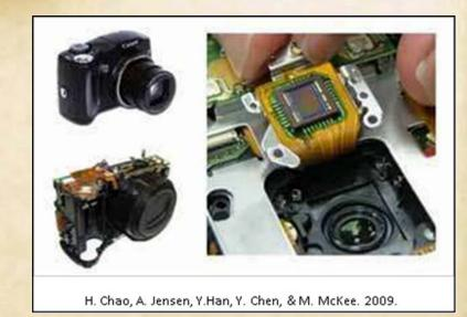
Commercial-off-the-shelf camera and image sensor. Camera could support Coastal Blue Band by replacing the visible light filter with a custom (400-450nm) narrow band filter
