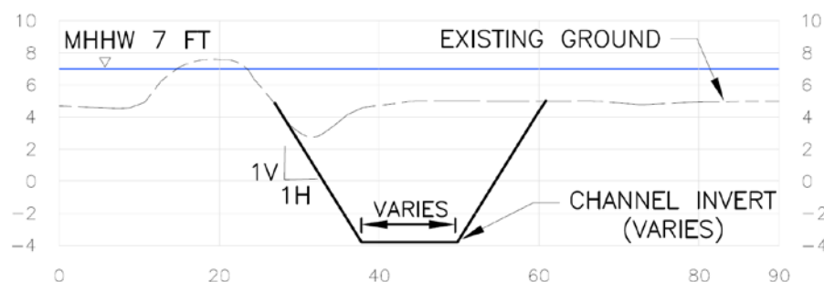
Figure 4.20. Proposed Pilot Channel – Typical Section
