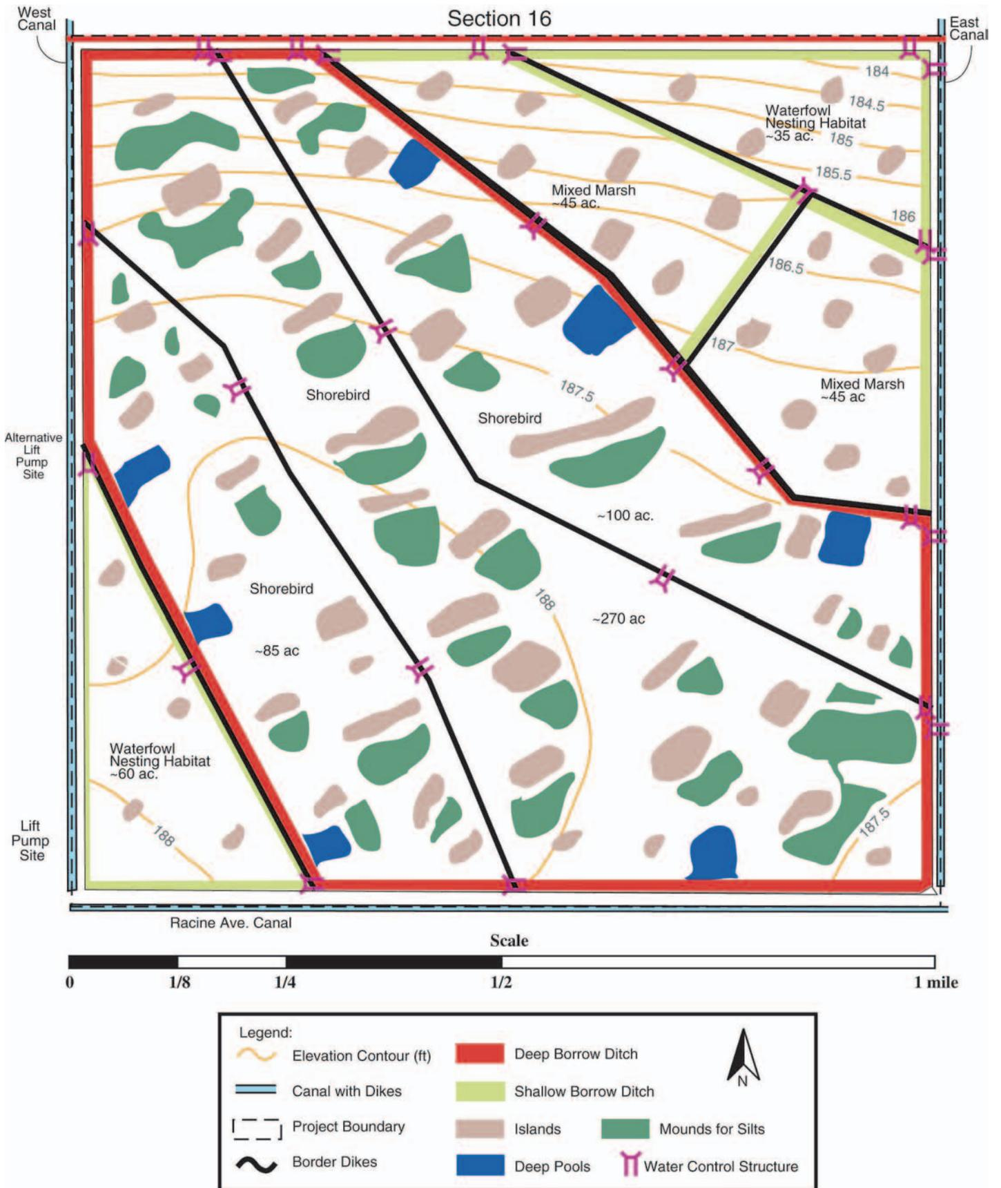
Figure 8: Successful Wetland Demonstration Project Design of a Managed Pond at Westlake Farms
