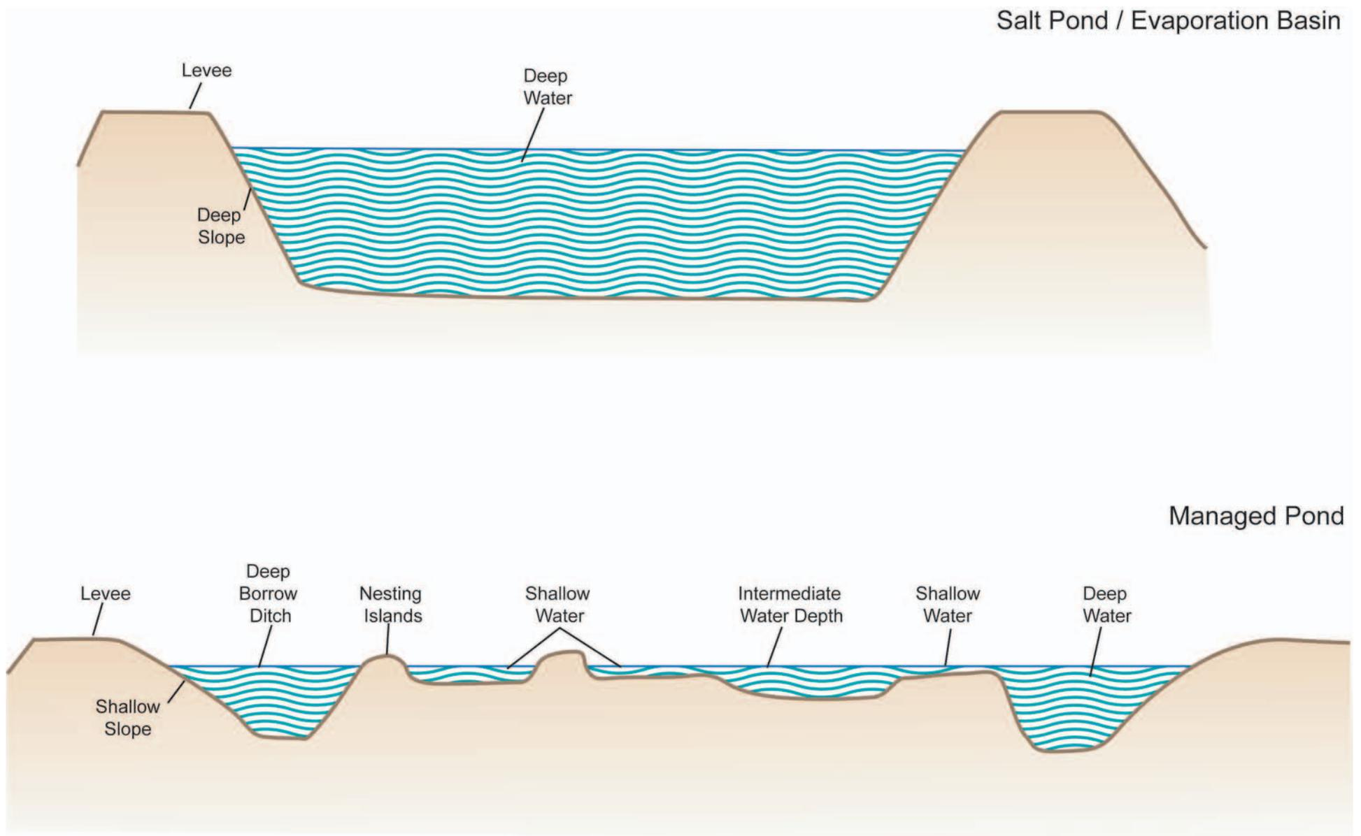
Figure 7: Conceptual Design of a Managed Pond to Maximize Avian Habitat
