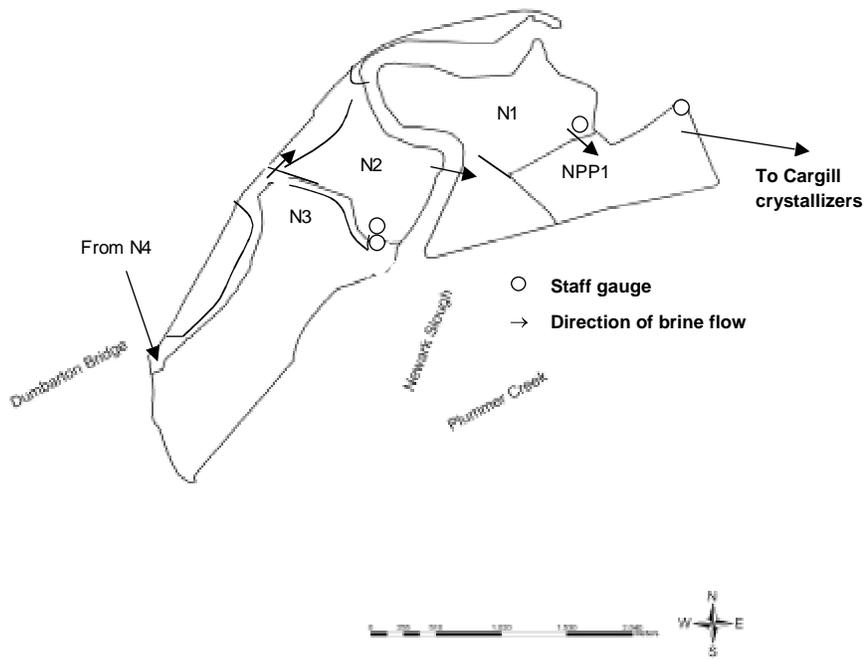
Figure 24. Dumbarton ponds diagram, showing staff gauge locations and direction of brine flow (reproduced from Murphy et al. 2007). Note: Flow of brines may vary depending on Cargill Salt’s business and/or operational needs.
