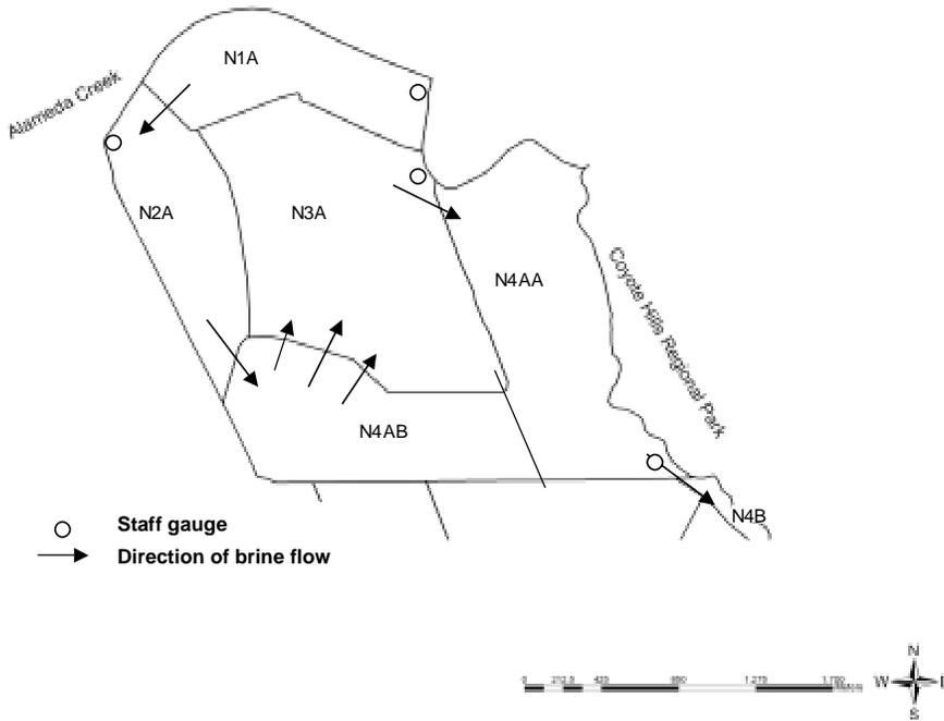
Figure 22. North Coyote Hills ponds diagram, showing staff gauge locations and direction of brine flow (reproduced from Murphy et al. 2007). Notes: Flow of brines may vary depending on Cargill Salt’s business and/or operational needs. Ponds N4AA and N4AB are considered a single pond by Cargill Salt and are collectively referred to as *Concentrator 4A*.
