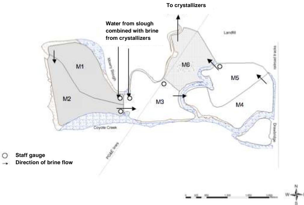
Figure 25. Mowry ponds diagram, showing staff gauge locations and direction of brine flow (reproduced from Murphy et al. 2007). Note: Flow of brines may vary depending on Cargill Salt’s business and/or operational needs.
