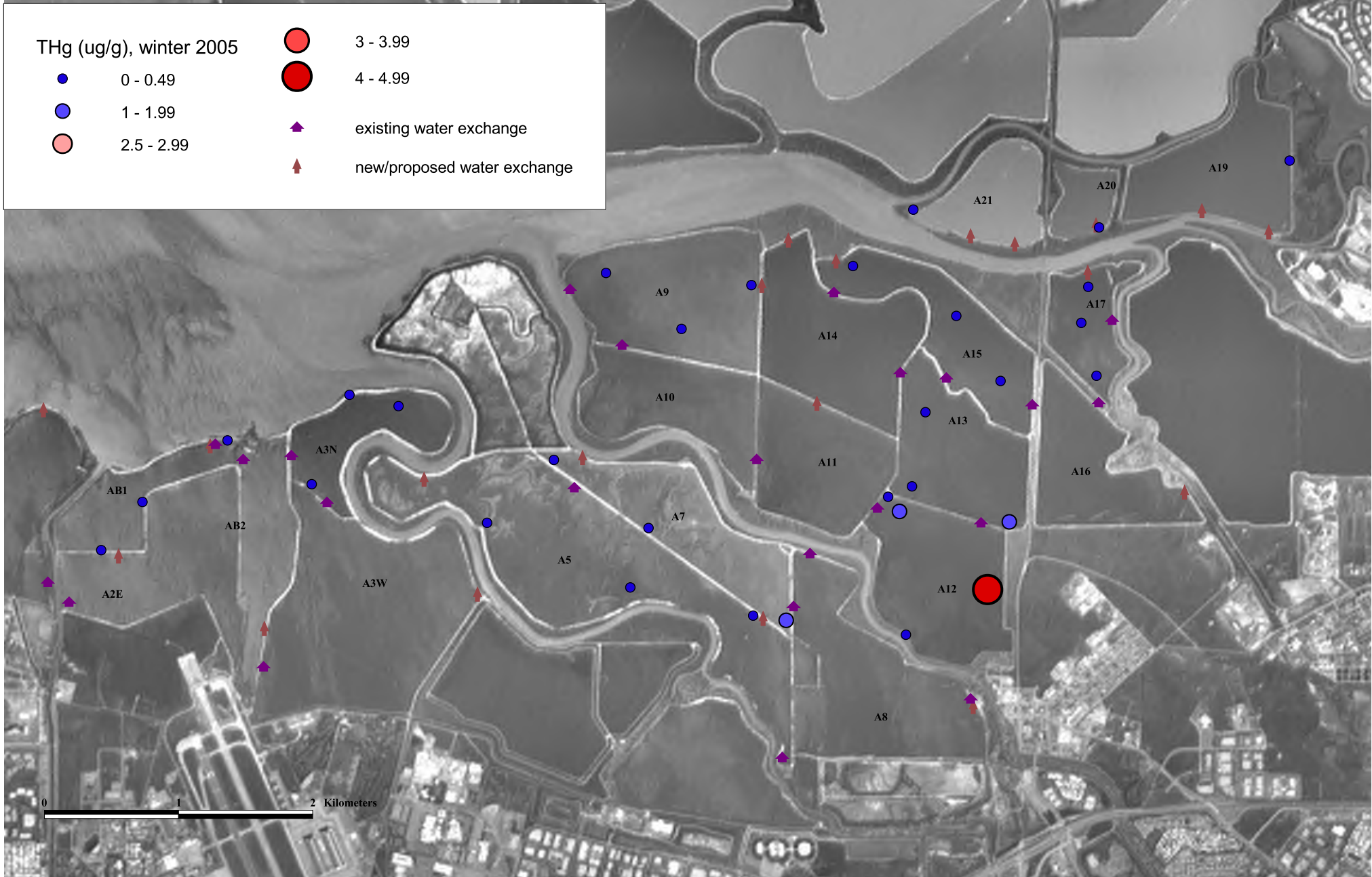
Figure 2. Concentrations of THg in surface sediment samples from Alviso Salt Ponds during February and March 2005. Points represent sampling locations except A19, 20, and 21 which were composite samples. Water exchange points taken from the Salt Pond ISP.
