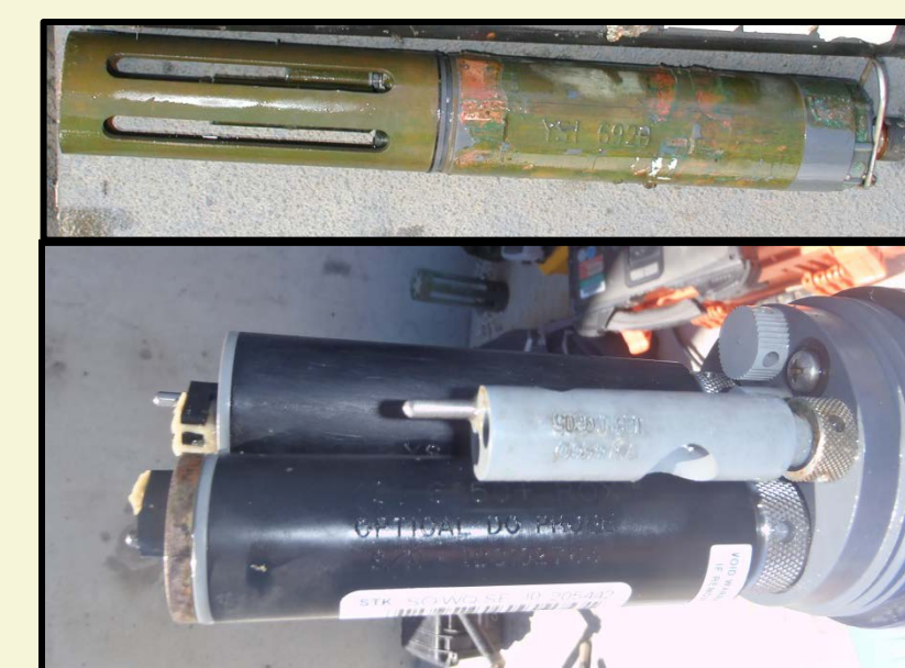
Figure 2. YSI Sonde, shown with sensor guard (top); close up of DO, turbidity, temperature, and specific conductance sensors (bottom).
