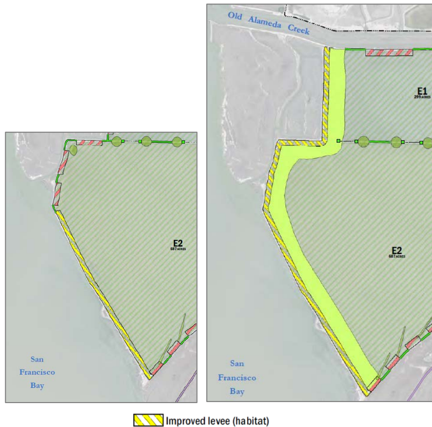
Figure 4.9. Plan of Bay Levee (Alt. C left, Alt. D right)
