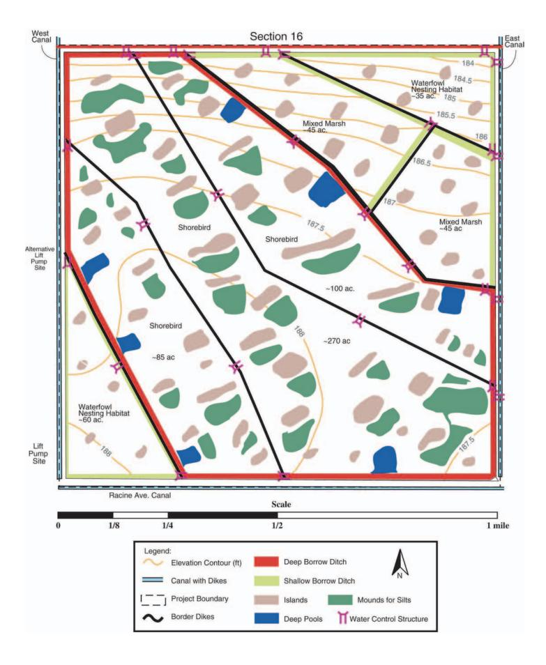
Figure 8: Successful Wetland Demonstration Project Design of a Managed Pond at Westlake Farms
