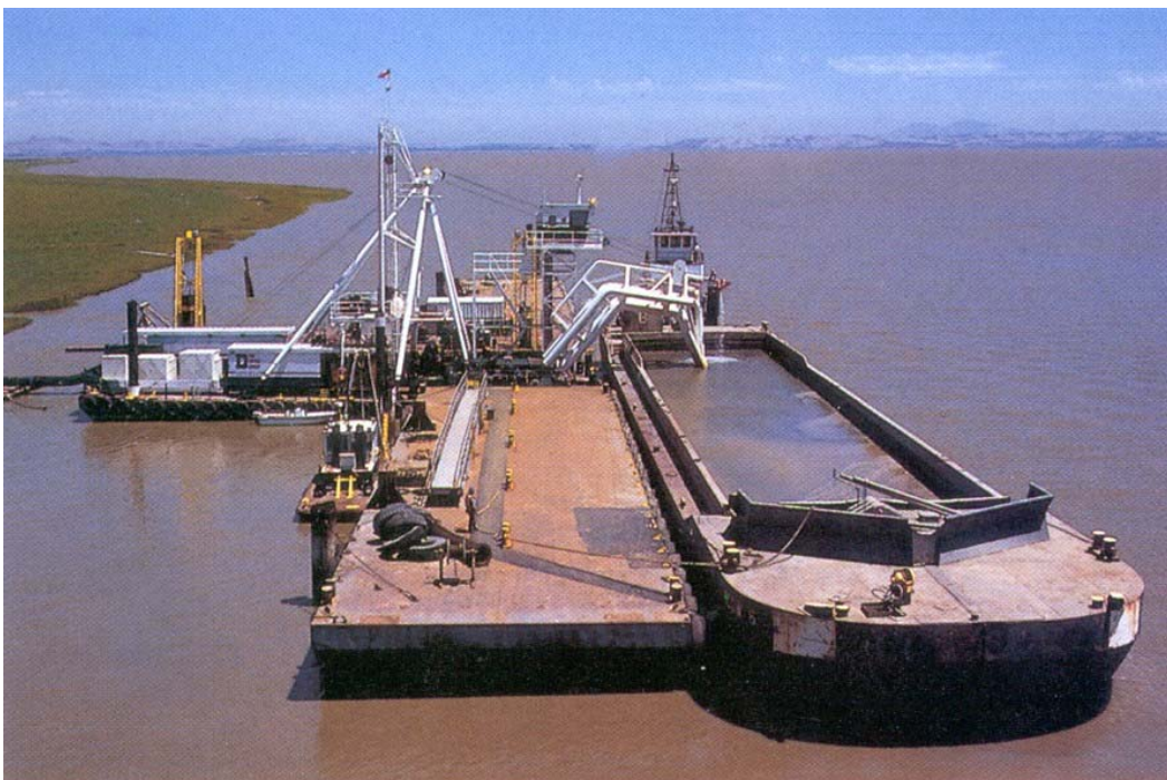
Figure 6-3 Liberty Offloader Pumping Dredged Material from a Scow
