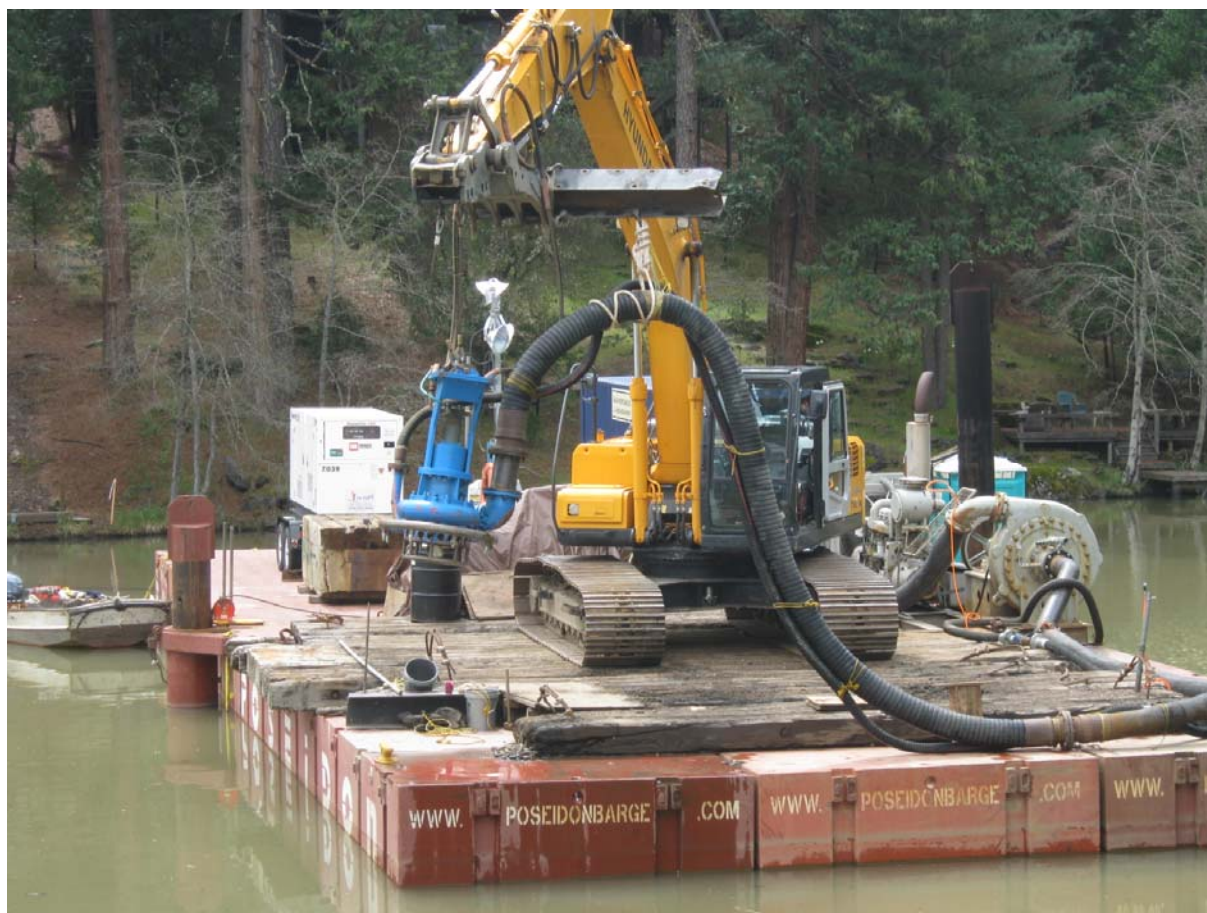
Figure 6-5 Submersible Pump Mounted on an Excavator
