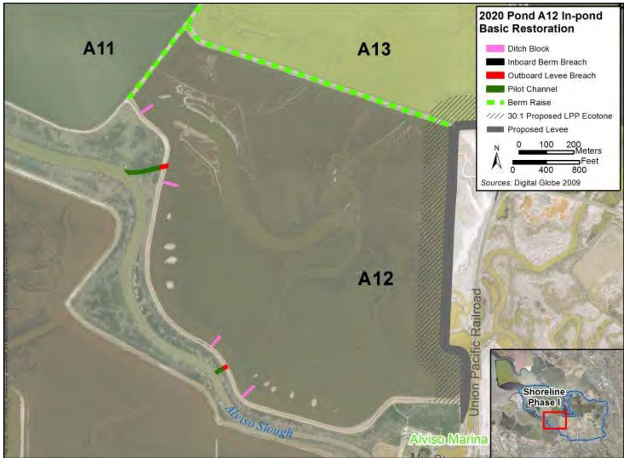
Diagram 2. In-Pond Preparation for Breaching of Pond A12.
