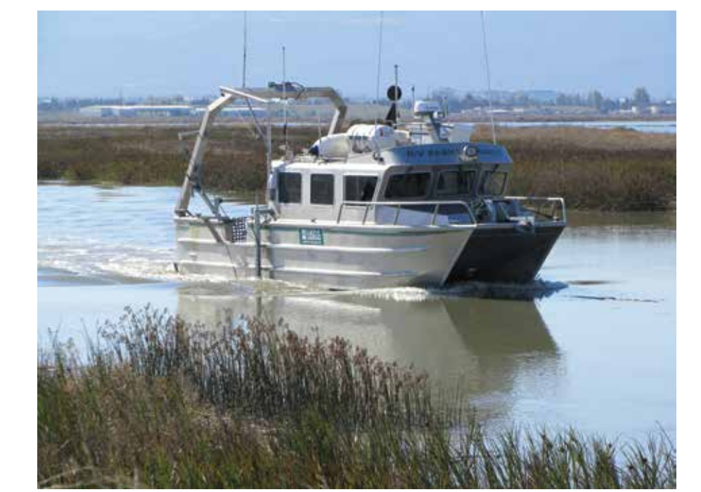
collecting swath bathymetry in Alviso Slough
