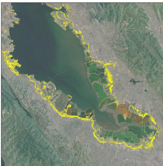
Raster output from the first order model was converted to vector polygons, simplified and adjacent polygons were merged. Final raster results were divided into “tidal and non-tidal based on “levee on” (tidal) and “levee off” (non-tidal) polygons provided by PRBO.
